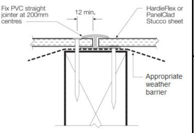
Figure 2: Sheet Joint on Timber Framing
