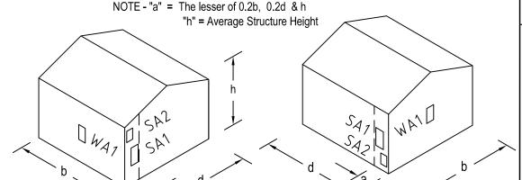
SA1 - KL = 1.5 - Side walls near windward wall edges within "a" of the edge SA2 - KL = 2.0 - Side walls near windward wall edges within "a"/2 of the edge
