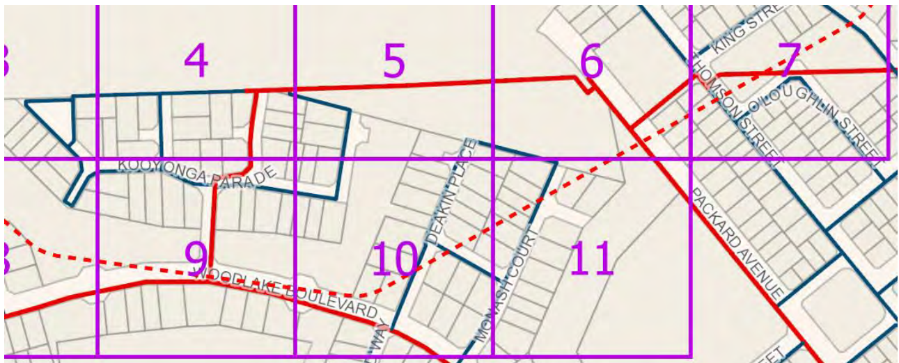
Figure 3-6 | Existing water Infrastructure Sourced from BYDA - Red Lines Show Trunk Mains and Blue lines show non-trunk infrastructure
