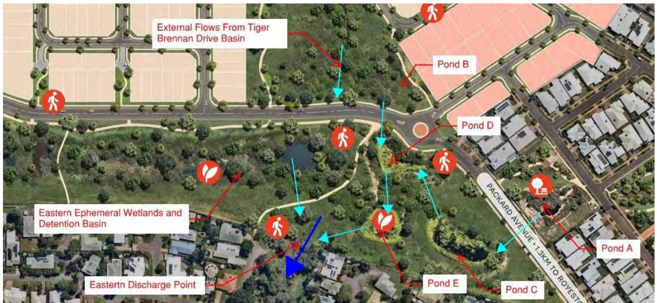
Figure 3-4 | Eastern Discharge Point and Stormwater Management
